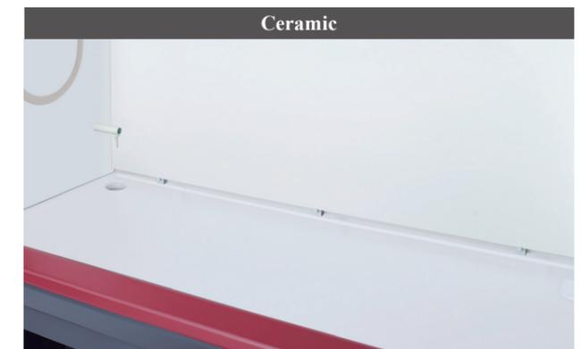
This work surface is a ceramic plate, whose main materials are silica sand and powder glass, fired at approx. 1100°C. In addition to superb chemical resistance, it offers incombustibility, anti-abrasion, non-conductivity, and other advantages.
