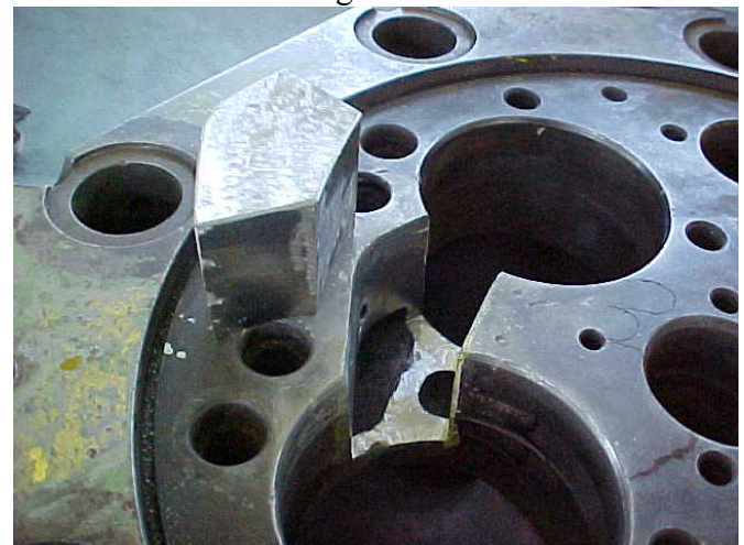
Fitting of Patch
