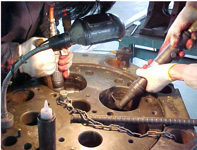
Stitching using Right Angle Tooling
