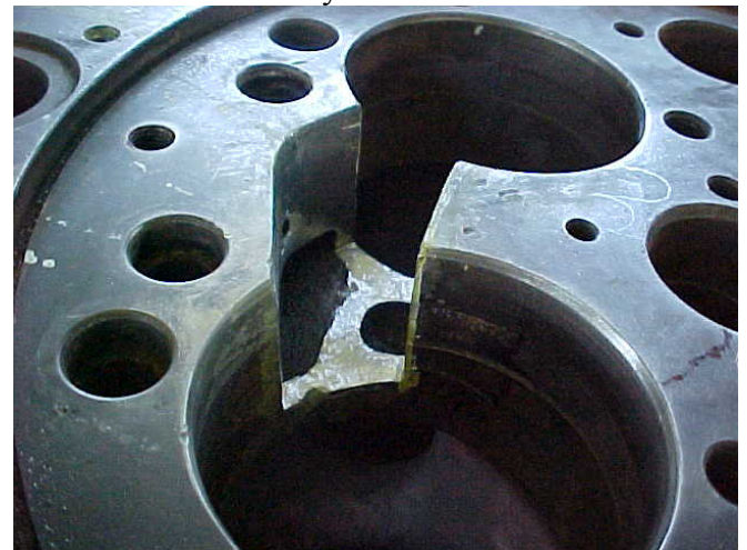
Grinding to Fit Patch
